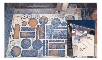
The alternate giveaway being cut, a set of rack and pinion gears
