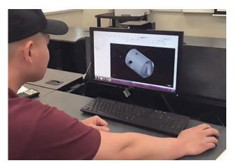
Student Pha Vang uses Mastercam to program a part that will be produced on a Haas CNC turning center.
