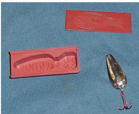
Students made an injection mold to create the plastic case for the fishing lure. Programmed by a CVTC student in Mastercam and produced on a Haas CNC mill. then allow them to be creative. Our injection molding equipment is pretty basic, but is very sufficient for our needs."
