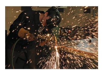
To check if the metal has reached its kindling point, slowly depress the cutting oxygen lever. If the cutting oxygen does not quickly burn through the plate, back off—otherwise, the result will be the shower of sparks shown here.
