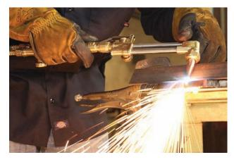
The major equipment manufacturers design equipment so that it is inherently safe to use. For example, this premium torch features built-in check valves and flashback arrestors.
