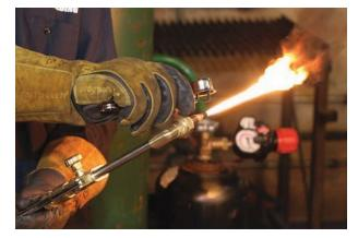
the acetylene valve 1/4-turn, and ignite the torch with a spark lighter, holding the lighter off to the side of the tip.
