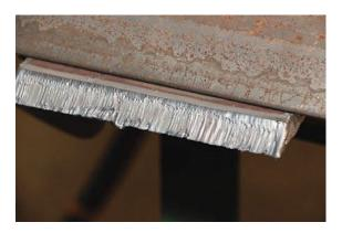
An oxy-fuel bevel cut—not bad for a student bevel cutting for the first time.
