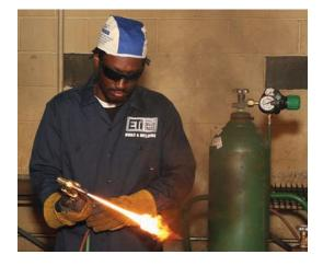
After lighting, the flame will generate a lot of soot and smoke. Continue opening the fuel valve until the smoke disappears.
