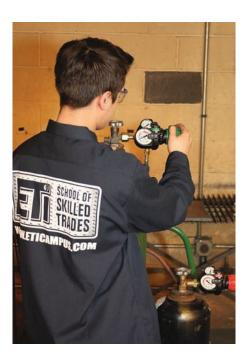
When setting gas flow rates, consult the manufacturer's tip chart. For the Victor 1-101 Series size #1 tip is used here, set oxygen flow at 30 to 35 CFH and acetylene flow at 3 to 5 CFH
