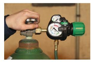
Open the oxygen cylinder valve all the way, as it is designed to seat in the fully open position.
