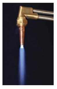
the oxygen level so that the flame shows both good pre-heat cones and a good cutting oxygen stream.
