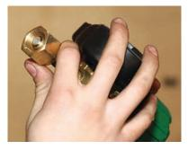
Visually inspect all threaded connections for signs of damage and contamination by grease, oil, or particles. Under high pressure and in the presence of oxygen, contaminants can easily combust.
