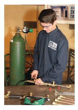
Use a wrench to tighten all metal-to-metal connections. This includes the regulator cylinder valve nut and hose connections. Hand-tighten connections involving an O-ring (such as between the torch handle and cutting attachment), as over-tightening could deform the O-ring.
