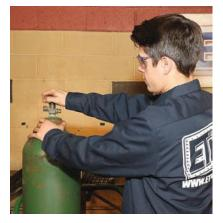
Before installing the regulator, briefly crack open the cylinder valve to blow out particles that might have been missed during visual inspection. Stand to the side or behind the valve, keeping your body out of the high-pressure gas flow.
