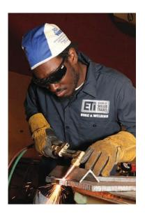
To bevel an edge, the operator uses a piece of angle iron and keeps it in place with another plate.
