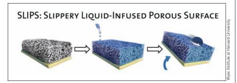
Fig. 1—The figures show openings that would be invisible unless you were looking at the object under an electron microscope. To infuse SLIPS, the outer layer of a metal or ceramic material would need to have micro-sized openings that serve as SLIPS wells to self-heal the outer coating if it is damaged.
