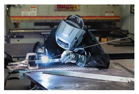
While GTAW is a slower process and therefore not typically used in high-production manufacturing, it is often a good choice in aluminum welding applications where productivity isn't as important but quality and appearance are critical.
