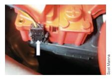
This is the electrical connection for a BMW Safety Battery Terminal, a pyrotechnic device that is designed to disconnect the battery in the event of an accident.
