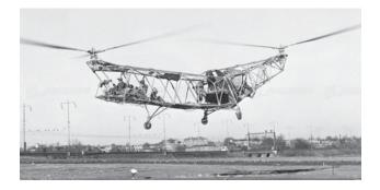
The Dogship in test flight without its fabric cover (to save weight)
