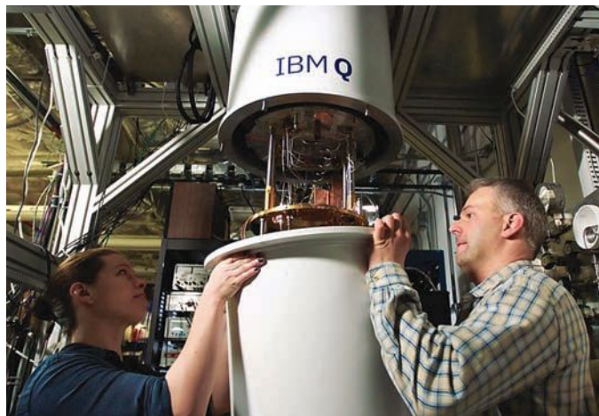
Photo 2—For the IBM dilution fridge to cool the qubits quantum processor to operating temperatures it is sealed into the container shown in this photo.
