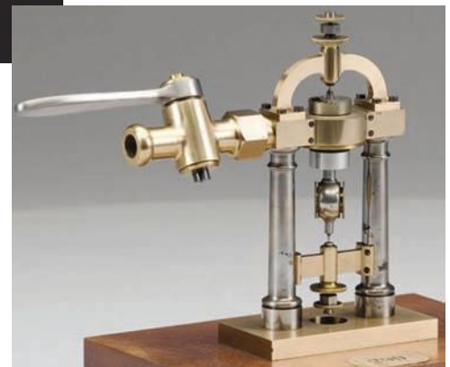
Right, a replica of Foucault's air turbine, with a rotating mirror at its center
