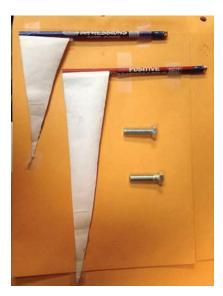
Photos 5 and 6—Showing how a screw is an inclined plane wrapped around a rod
