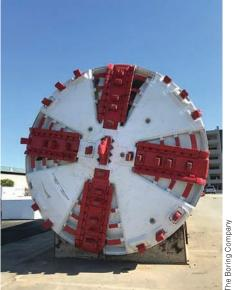
Photo 4 —Cutting end of Godot. It can cut through all kinds of rock and soil, and not get bogged down in mud or other impediments that clog other machines.
