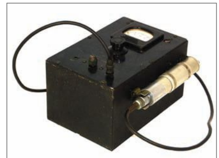
Geiger counter built at Harvard University in the 1940s
