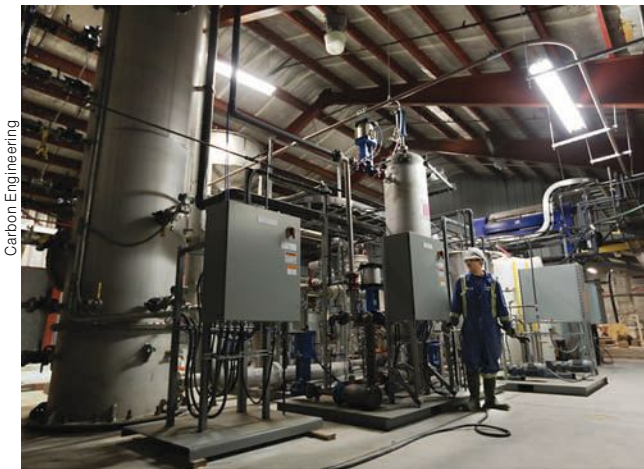
Photo 3—The reactor is one of the many machines that helps process and convert the CO 2 into a fuel.
