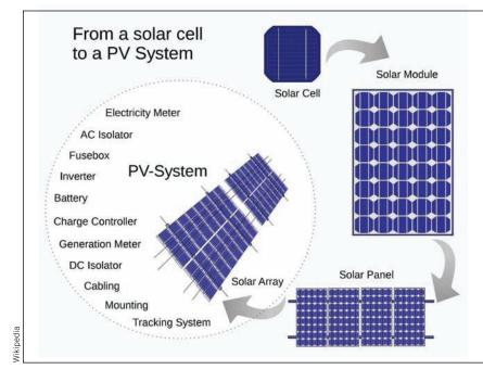
Fig. 2–PV cells are combined into modules then into panels to form end products.
