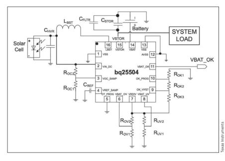
Fig. 5—Application circuit for energy-harvested battery charging using TI power management IC.
