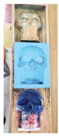
Right, another object cast in a two-part mold made from a 3D-printed model. Notice the "nobbies" added to align the two sides of the mold, and sprues added to allow the material to be poured into the mold, and air to escape while the material is poured in.
