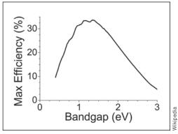
Fig. 3—Shockley and Queisser's calculation of maximum efficiency against band gap for single-junction PV cell semiconductors. Silicon has a band gap of 1.1 eV.
