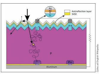
Fig. 1—Single-junction PV cell operation: Photons of appropriate energy liberate electrons, which cross the semiconductor junction and generate a potential difference.
