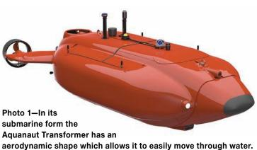
The Aquanaut Transformer is real, and it shape-shifts between a submarine and an Aquanaut robot (Photos 1 and 2). Its submarine shape allows it to quickly move through the water to get where it needs to be. Once there, it shape-shifts into a very powerful humanoid robot which can perform all kinds of underwater construction tasks.
