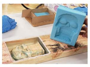
puter. Many of the same files that can be used with a 3D printer can be 3D carved on a ShopBot, and the resulting model can be used to create molds to aid in the production of many copies.
