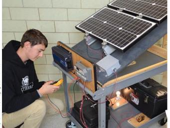
Using energy converted using a portable photovoltaic system, a Bridging Communities student determines the load on the circuit powered by the 12 V battery.
