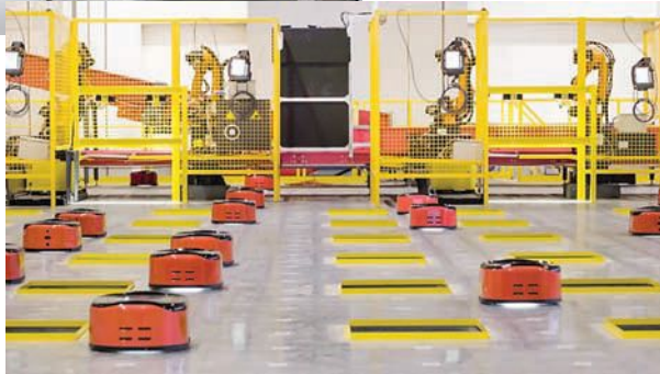
Photos 4 and 5—An AI logistics system controls robotic arms, conveyor belts, and automated trolleys throughout this fulfillment warehouse.
