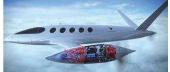
drives its engines. Its three engines are actually three very powerful electric motors. Each of these supersized motors has the same working parts as the motors you find in your home, a stator that creates the magnetic field that turns electrical energy into mechanical energy, and a rotor that spins the propeller (Photo 2).
