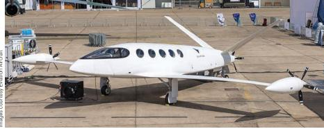
Photo 1—The Alice aircraft is powered only by its lithium ion batteries.
