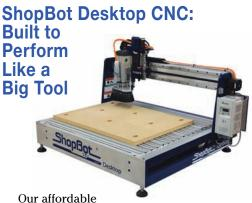
ShopBot Desktop, with a 24" × 18" cutting bed, is a digital fabrication powerhouse. The Desktop delivers engraving level precision and has the power and rigidity to machine parts from wood, plastic, aluminum, and other materials. Not only can it perform a wide range of prototyping and production projects, the Desktop is also an agile platform to support your growing digital fabrication interests and needs.
