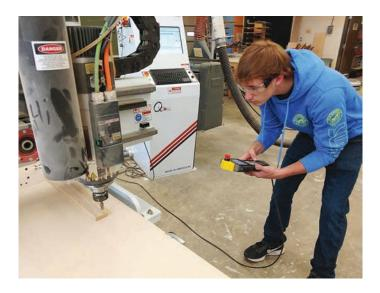
work, students will have the opportunity to use the CAD/CAM software and the CNC router to create more than the usual round 'dots' you see on the average fret board. The materials for these inserts, such as stars and unique icons, will also be programmed and machined on the router."
