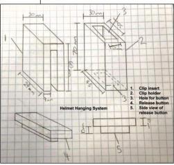
a storage system that used elastic straps mounted to the walls and roof of a fire truck. Another team of Tobin, Eliza, and Peter utilized Autodesk Fusion 360 to design a simple yet effective clip system for hanging fire helmets that often fall off the wall inside the fire truck. Those students, along with others, exported their designs as STL files, sliced them using Cura software, and 3D printed them on inexpensive but effective 3D printers.
